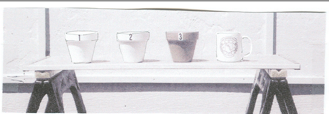
Figure 5. Small clay flower pots filled with water: #1 lime wash; # 2 enamel paint; # 3 unpainted clay color. Pots exposed to full sun with for three hours in late afternoon.
